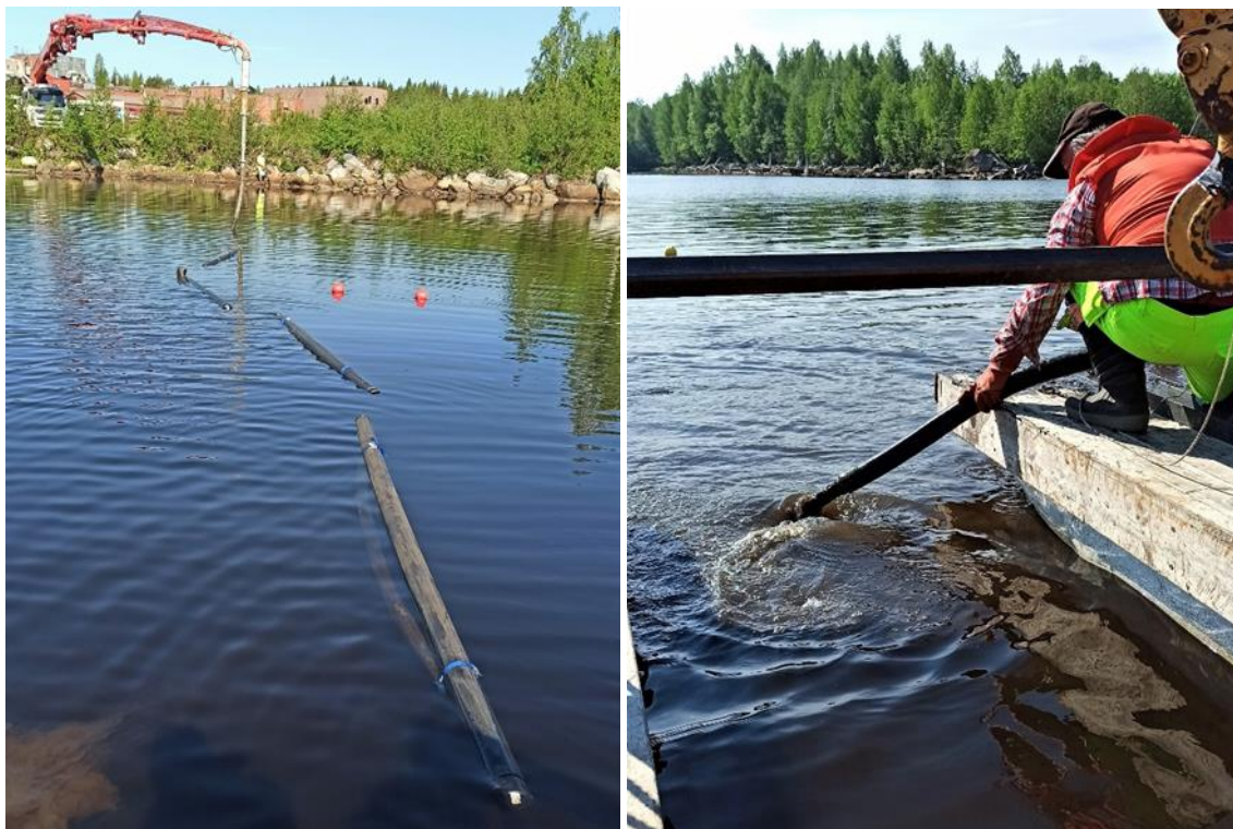
Figure 5 A tube was mounted to the crane lorry to transport the biochar mixture to the test area (a) and the biochar-mixture was spread in the water from the floating dock (b) (Flodin, 2021).
