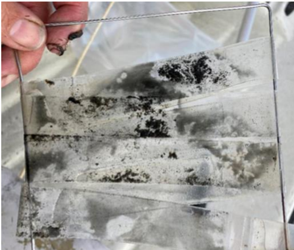
Figure 4 The adsorbing membranes attached to the samplers (Flodin, 2021).
